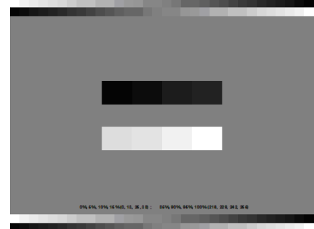
Fig. 1. Pattern (SET01S50) to set up the front-projector.
