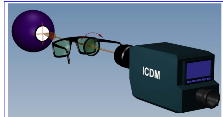
Fig. 3. Testing glasses polarization quality using a uniform source and a good linear polarizing filter.
